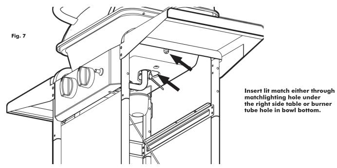
If any or all Burners fail to light after three or four attempts following Steps 3-4, turn all Control Knobs to the "Off" position and close the LP Gas Cylinder value to dissipate any accumulated gas. Wait five minutes; then repeat the lighting procedures.
